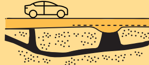
Voids Bridging and Protection from Subsidence
