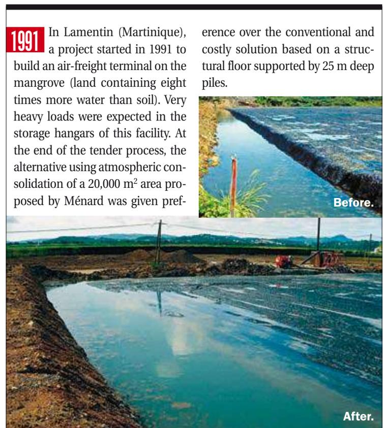
**1991** In Lamentin (Martinique), a project started in 1991 to build an air-freight terminal on the mangrove (land containing eight times more water than soil). Very heavy loads were expected in the storage hangars of this facility. At the end of the tender process, the alternative using atmospheric consolidation of a 20,000 m<sup>2</sup> area proposed by Ménard was given preference
