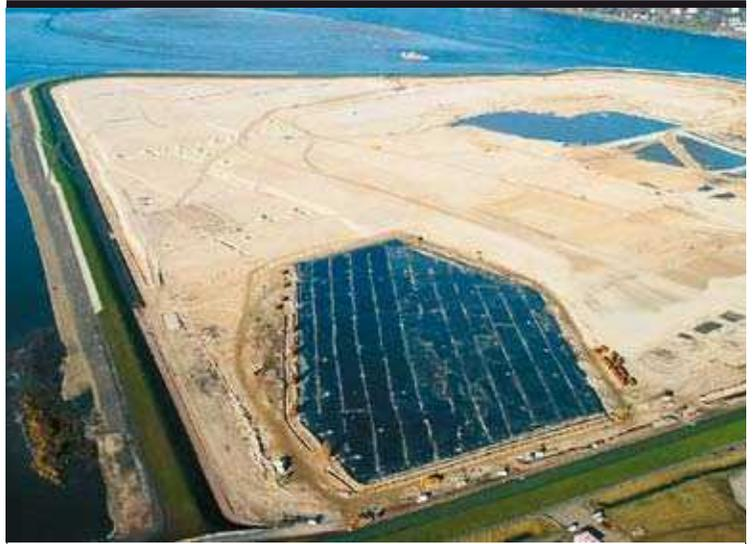
**2001** In Hamburg (Germany), the Airbus A380 assembly site is built on 140 ha of land reclaimed from a dead branch of the Elbe consisting of muddy deposits. To isolate
